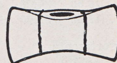
DOUBLE BIT EYE AND BLADE ELECTRICALLY FUSED TOGETHER
